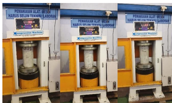
Figure 6. Compressive Strength Test
