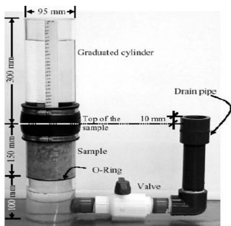
Gambar 2. Alat uji permeabilitas beton porous (ACI 522R-10)
