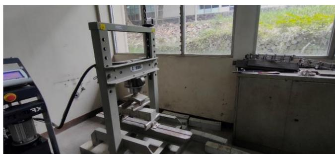
Gambar 3. Alat *bending machine*
