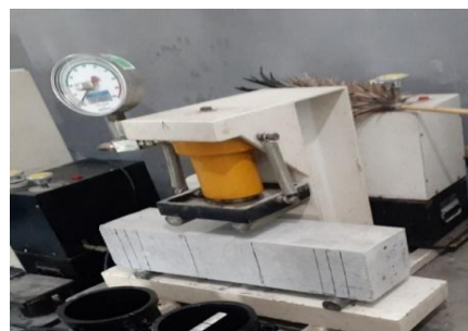
Gambar 3. Proses uji kuat lentur beton fast track FS 45.
