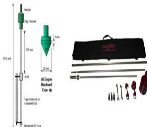
Gambar 3. Alat uji Dynamic Cone Penetrometer
