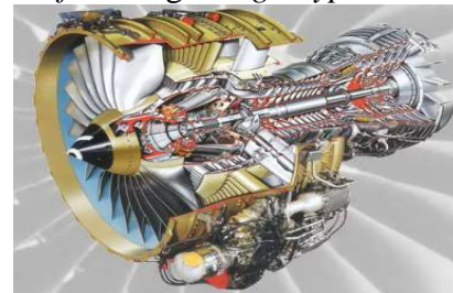
Gambar 2. Penampang melintang engine CFM56-7B
