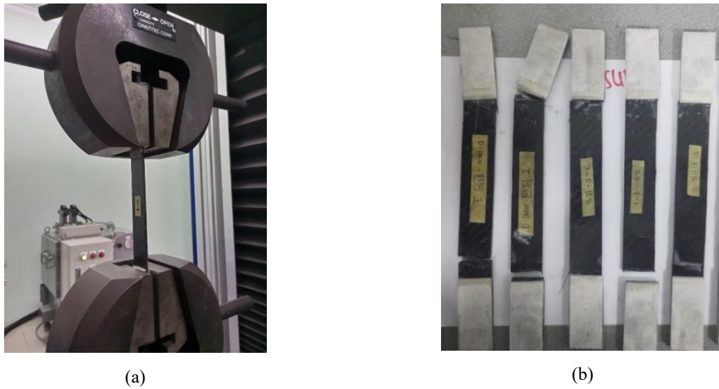
Figure 4. (a) Tensile Test process, (b) Example of tensile test specimen
