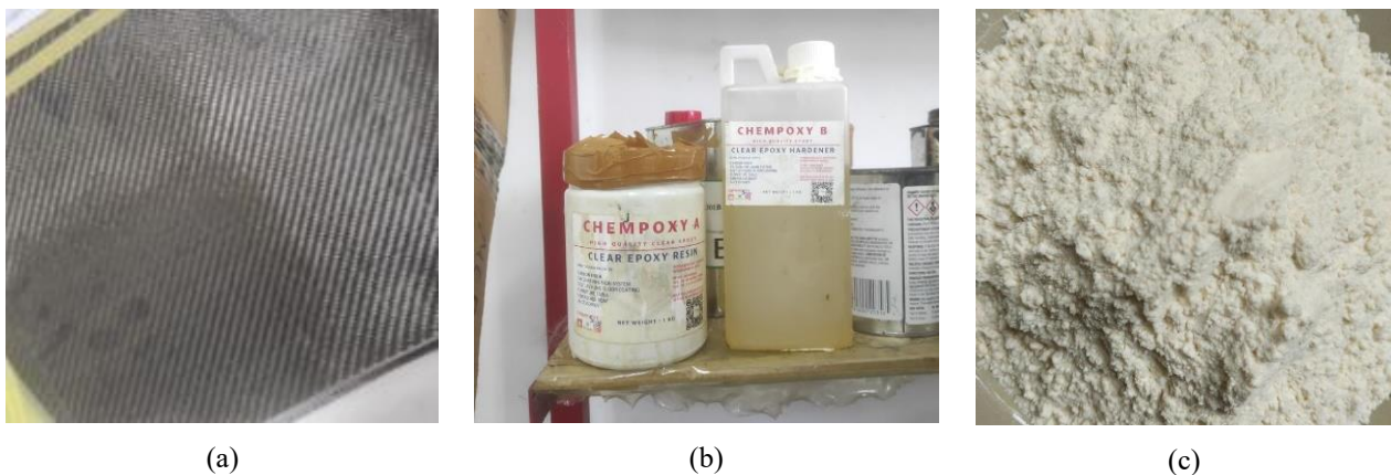
Figure 1. Material Used: (a) Carbon Fiber Twill 2x2, (b) Epoxy and Hardener, (c) Palm Flour
