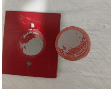
Figure 4. Condition of the Specimen After Adhesion Strength Testing
