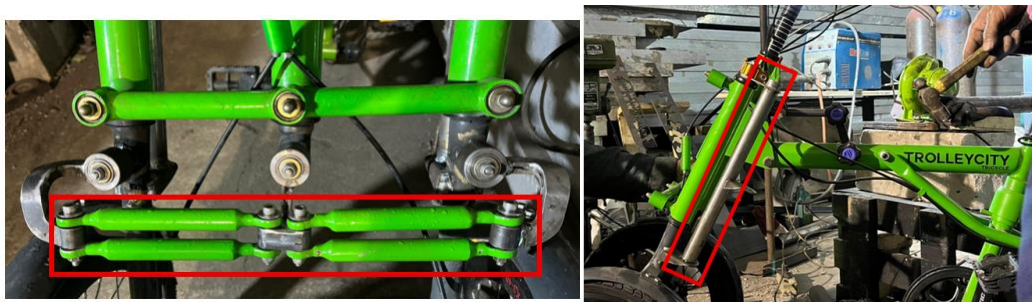
Figure 8. Double link on bracket (left) and gas spring mount (right)
