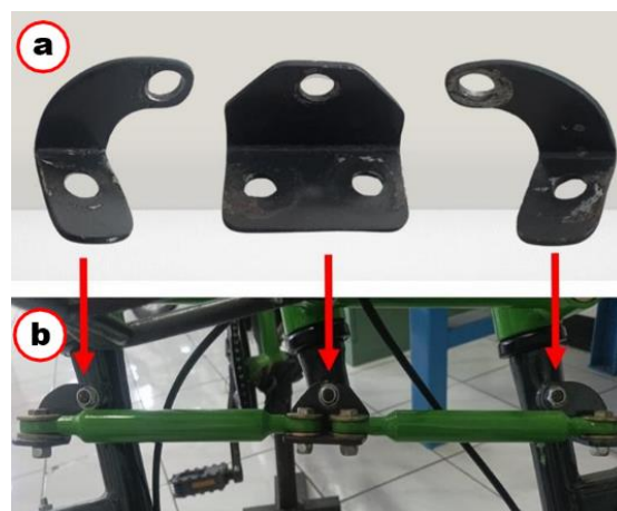
Figure 2. (a) Side and centre bracket (b) Condition of the bracket when installed
