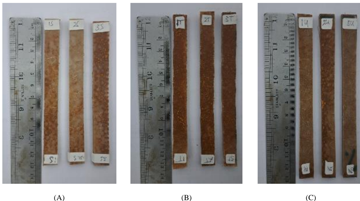
Figure 4. Burn Test specimen, (A) 2% Clay : 28% SR : 70% PP, (B) 4% Clay 26% SR : 70% PP, and (C) 6% Clay : 24% SR : 70% PP
