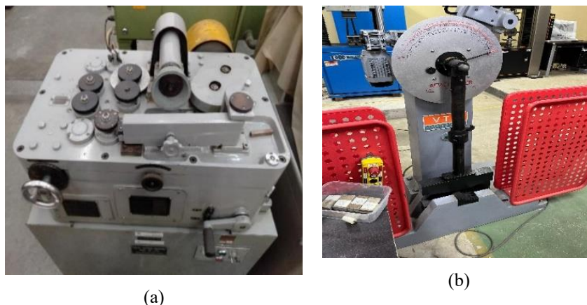
Figure 2. Experimental testing machine (a) Ogoshi wear testing machine type OAT-U, (b) Charpy impact testing machine
