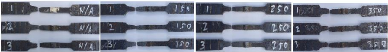
Figure 3. Fractured tensile specimens at different preheating temperatures
