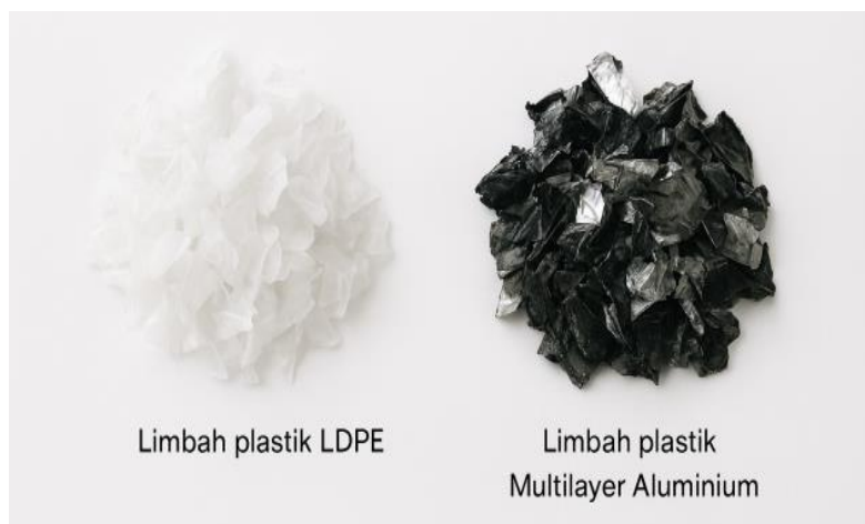
Figure 2. Raw Materials Used in the Study: LDPE Plastic Waste and Multilayer Aluminum Plastic Waste
