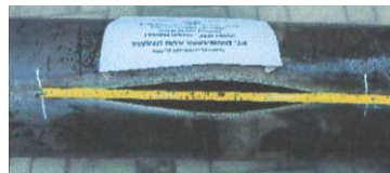
Figure 2. Burst pressure experiment results
