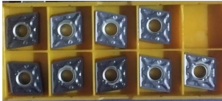
Figure 1. Insert Carbide CNMG 120404 - MA
