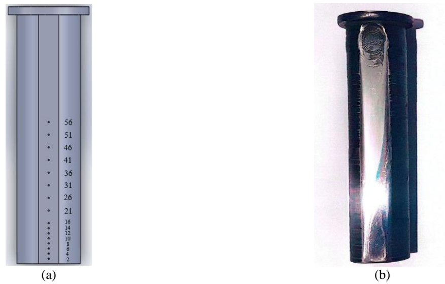
Figure 3. Jominy specimen: (a) design, (b) actual specimen
