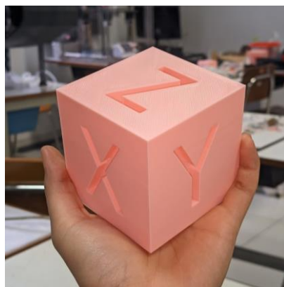
Figure 3. Printing specimen of 80 \times 80 \times 80 mm calibration cube for 5-hour endurance testing
