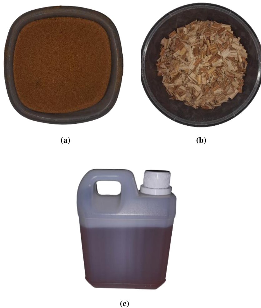
Figure 1. (a) Wood Sawdust, (b) Moringa Fruit Skin Fiber, (c) Unsaturated Polyester Resin
