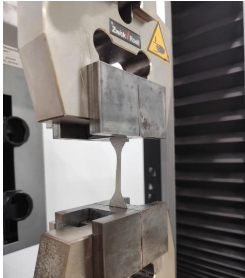
Figure 3. Photograph of the specimen during the interlayer adhesion test
