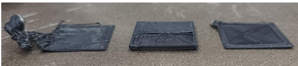
Figure 9. HIPS specimen forming failure
