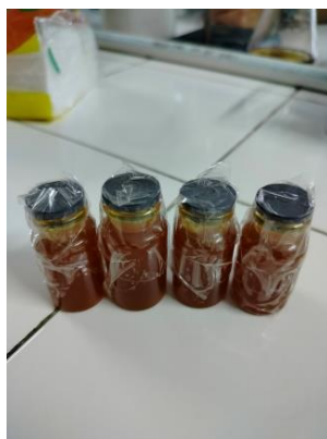
Figure 4. Biolubricant derived from castor oil.
