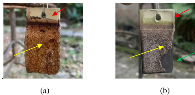
Figure 8. (a) Specimen after immersion (b) Specimen after cleaning and drying
