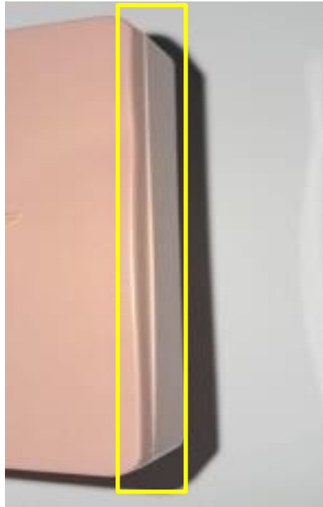
Figure 1 Gap that occurs in the product when installed with the cover
