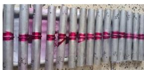
Gambar 5. Proses pengujian NDT *dye penetrant test*
