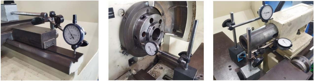
Gambar 3. Proses Pengukuran Geometri Guide Ways, Spindle, dan Tailstock
