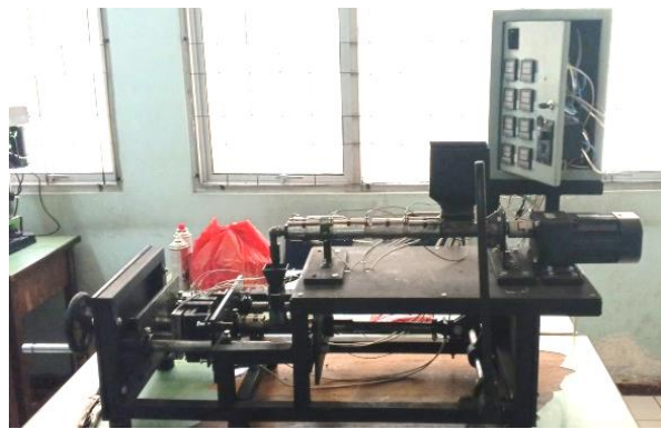
Gambar 1. Prototype mesin injeksi plastic molding manual double barrel kapasitas 5 TF
