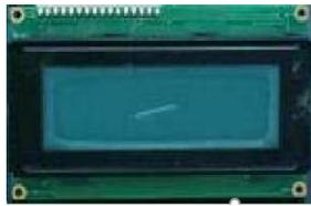
Gambar 4. LCD 20x4
