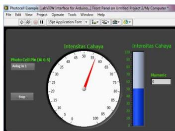
Gambar 7. Front Panel Rancangan LIFA Pengukur Intensitas Cahaya
