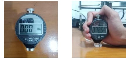
Gambar 4. (a) Durometer digital shore A (b) Proses pengujian spesimen
