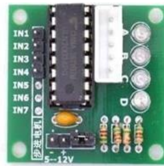
Gambar 5. Motor driver ULN2003A
