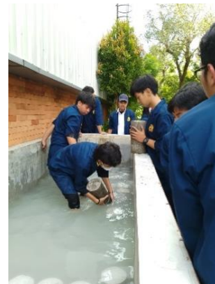
Gambar 3. Proses Curing Slinder Beton
