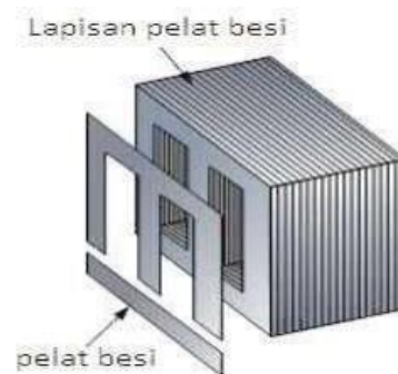
gambar.2.3. Inti Besi Transformator
