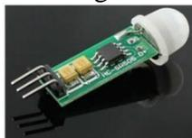
Gambar 5 Modul Sensor PIR
