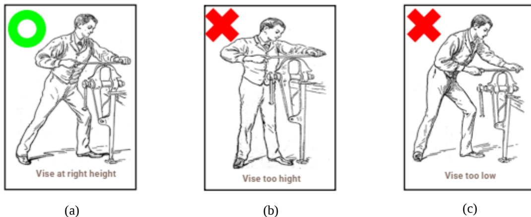
Figure 2. Ergonomic and non-ergonomic position in bench work: (a) Vise right at height, (b) Vise too high and (c) Vise too low
