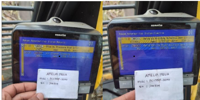
Gambar 4. Pengecekan monitor panel
