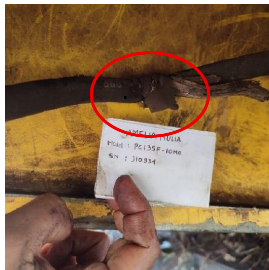
Gambar 3. Hose fuel return to tank terjepit
