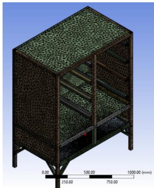
Figure 2. Generated mesh of the cabinet dryer model with applied element sizing.
