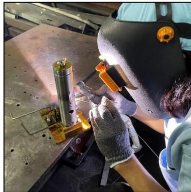
Gambar 5. Penggunaan Welding Fixture Inner Joint
