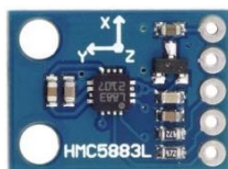
Figure 2.1 HMC5883L Compass Sensor Module (Ecadio, 2016)
