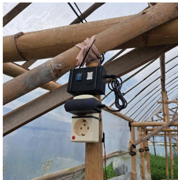
Fig 7. Implementation of the ChrysoSmart sensor node installed in the chrysanthemum greenhouse
