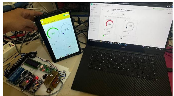
Fig 7. Testing of the IoT-based monitoring and control system in laboratory
