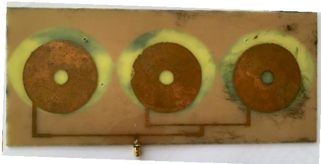
**Figure 3. Structure of Antenna Array 3X1-LoRa transceiver** Structure of Antenna Array 3X1-LoRa transceiver: (a) perspective view; (b) Side view. The structure consists of two layers: the lower layer of electronics and the upper layer of the antenna, which are connected through the signal vias.
