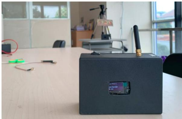
Figure 17. The measurement is done through two LoRa transceivers, with the first being the sensor tag and the second being the reader.
