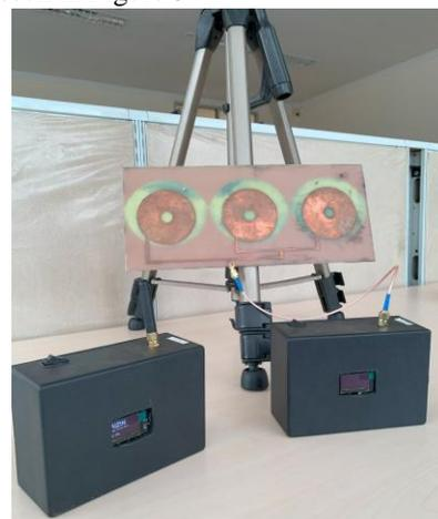
**Figure 6. Prototype of the 3x1-LoRa Antenna Array transceiver board**
