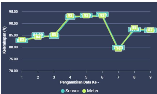
Fig 24. Comparison Results of Humidity Sensor and Hygrometer
