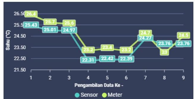
Fig 22. Comparison Results of Sensors and Thermometers
