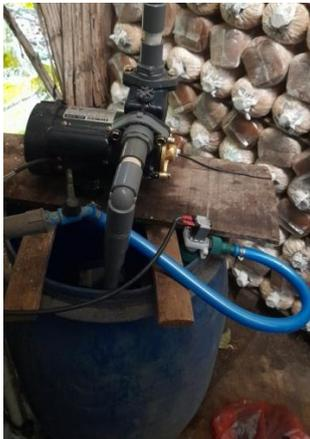
Fig 8. Location of Solenoid Valve and Water Pump
