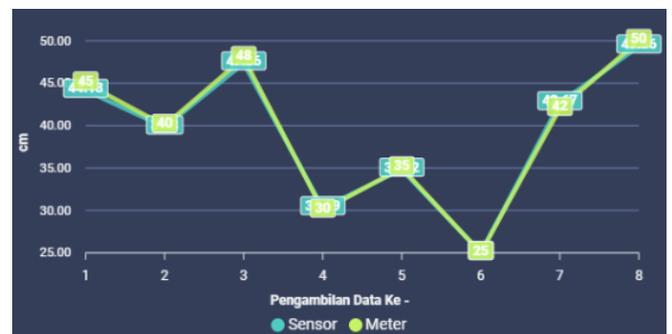
Fig 26. Comparison of Water Level Sensor and Meter
