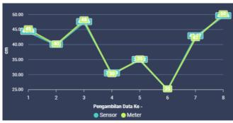
Fig 26. Comparison of Water Level Sensor and Meter
