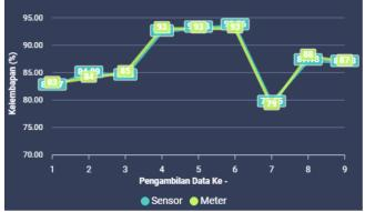
Fig 24. Comparison Results of Humidity Sensor and Hygrometer
