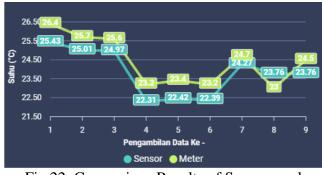
Fig 22. Comparison Results of Sensors and Thermometers
