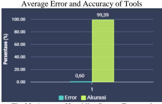
Fig 23. Average Humidity Sensor Error and Accuracy
