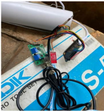
Figure 2.4. Measurement pH, Temperature, Turbidity
