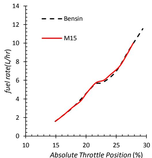
Gambar 9. Grafik *absolute throttle position versus fuel rate*
