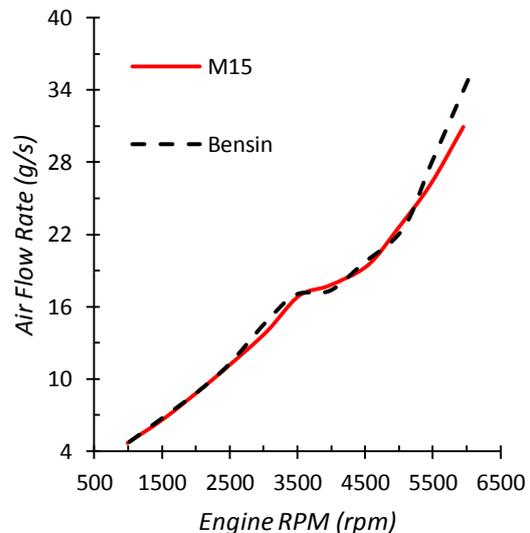
Gambar 12. Grafik engine speed versus air flow rate
