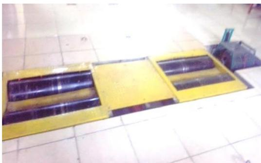
Gambar 5. Chassis Dynamometer
