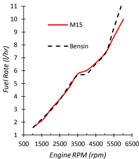
Gambar 13. Grafik engine speed versus fuel rate
