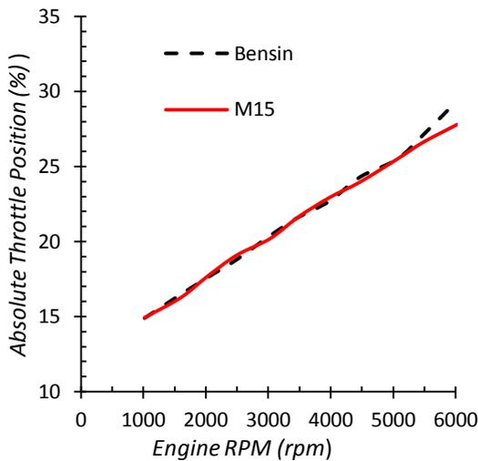
Gambar 10. Grafik engine speed versus absolute throttle position
