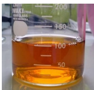
Fig. 2. Crude lipase extract obtained from oil palm mesocarp
