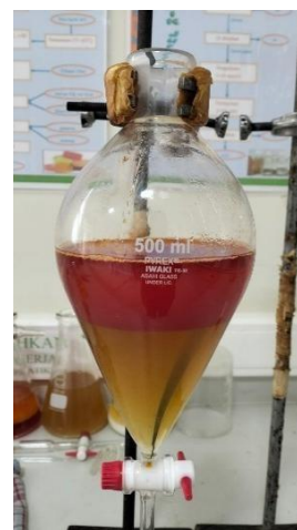
Fig. 4. Phase separation of free fatty acids and glycerol after enzymatic hydrolysis of waste cooking oil
