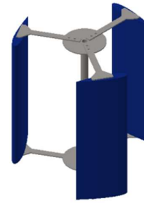
Figure 3.4 H-Type Darrieus Turbine With NACA Blades 0018
