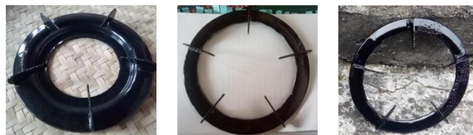
Gambar 1. Perancangan Grid Diameter Lubang 0.4; 0.6; 0.8 cm
