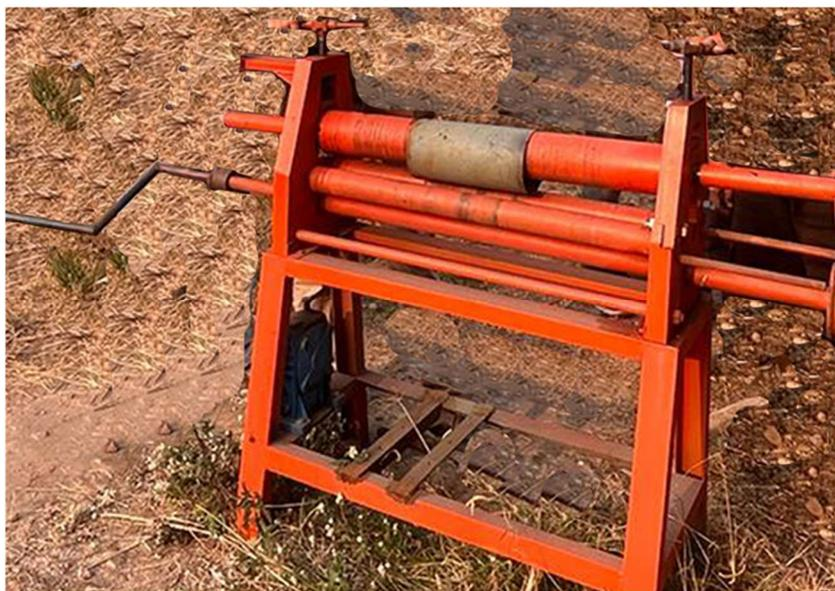
Gambar 2. Mesin roll bending
