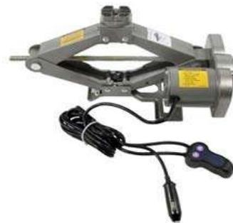
Gambar 2.2 Dongkrak Gunting Elektrik
