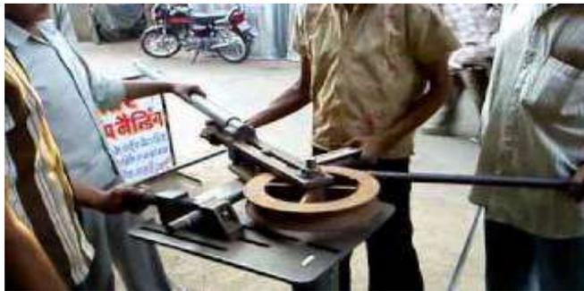
**Gambar** Alat *Rolling* Pipa Konvensional
